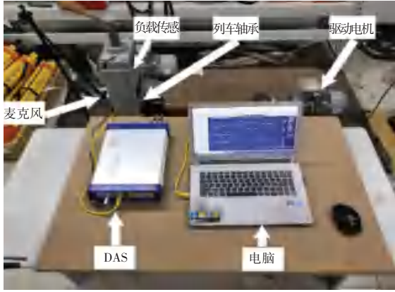
(a) 轴承实验台 (a) Bearing bench
