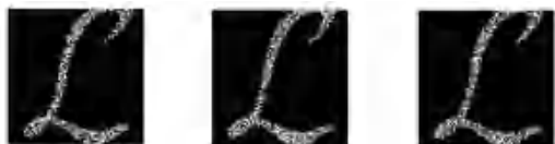
(a) 斑点噪声 (b) 高斯噪声 (c) 椒盐噪声 (a) Speckle noise (b) Gaussian noise (c) Salt and pepper noise
