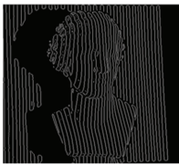
(c) 使用方向可控滤波器及基于矩恒定原理得到的阈值检测的结果 (c) Threshold detection results based on the principle of moment constant and steerable filter
